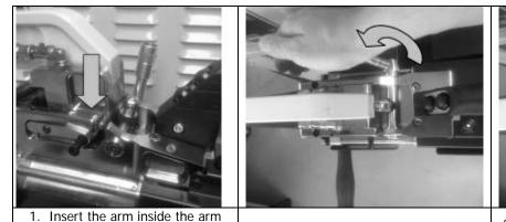
2. Turn lever E towards the front of the clamp to push the arm in position.
