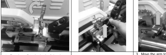
1. Turn lever E to the back of the clamp and place it vertically.
