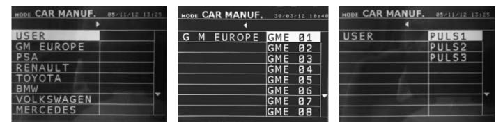
User programmed welding spots can be recalled by selecting USER in the list of car manufacturers. The welding spots can be programmed using the welding spot programming module in the GYSPOT software.
