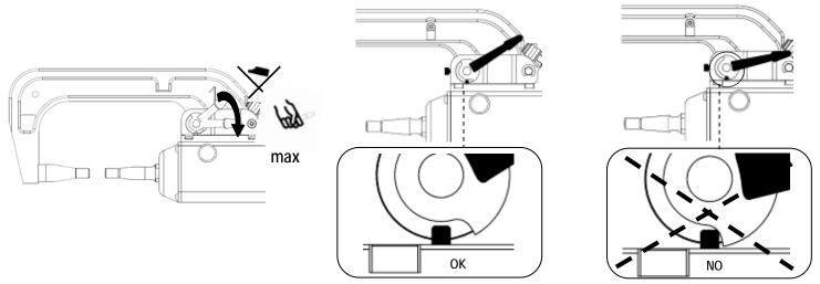
Warning: Clamp and arm may be damaged if the lever is not tightened properly.
