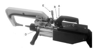
A button : close the clamp and weld
