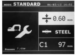
The sev is used to enter the clamp adjustment mode. The clamp adjustment mode allows the user to close the clamp and apply the programmed force on the electrodes without any current flowing. This mode is used to adjust the arms. The clamp will remain closed as long as the button remains pressed; this allows the user to check the alignment of the electrodes and positioning of the caps.
