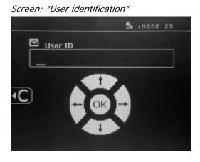
The « left » and « right » arrow keys move the cursor within the field. The up and down arrow keys scroll through letters or figures. Press Esc to erase the field. The Mode button changes the field to modify playback.
