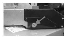
The screw shown opposite ensures secure attachment of the copper cable which carries current to the clamp. It is recommended that screw tightness is checked every month to prevent irreversible damage inside the clamp.
