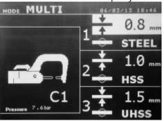
Using The up and down button (key definition diagram, (5) ) allows selection of the parameters for each sheet. When the parameters for a sheet are highlighted, the sheet thickness and type of steel can be adjusted using the + and - keys (key definition diagram, (3)).
