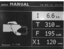
This mode allows the user to manually select the welding parameters, for example when following instructions from a manufacturer . The settings proposed by default in the manual mode correspond to the settings automatically selected by the standard mode (thickness and type of sheet, electrode force, arm).
