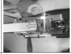
3. When lever E is pushed forward to the stop position, the arm is inserted correctly into position.
