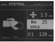
The auto mode is identical to normal mode except that the user enters the yield strength of steel. The Ys may be found using a durometer such as Gysteel Vision
