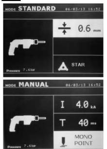
• In standard mode, the gun can weld a maximum of 1.5mm thick sheets. When using the gun, the operator can choose between several tools (single spot, carbon shrinking, star welding, studs, rivets, washers, stitches). The tool selection is made with + and - keys.
